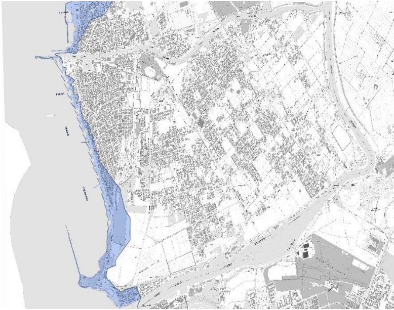
Fig. 1. Areas at risk of flooding due to sea level rise in Isola Sacra – Fiumicino (blue polygon). SLR data compared to today: 63 cm; time horizon: 2100.
